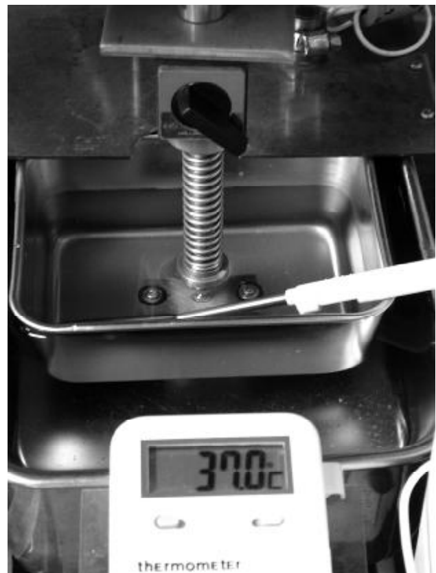
Fig. 3. Specially constructed jig was connected to a load cell of fatigue machine. Demineralized water was warmed up to 37 C by 38 C water circulating outside the bath
